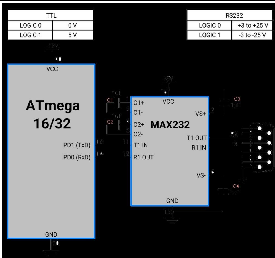
ATmega16/32 Serial Interface Connection Diagram
